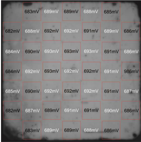
Figure 9: PL image after laser ablation on n-type TOPCon measured from the non-laser ablated side. The iV_{oc} values are determined by QSSPC measurement. The red fields with black values reveal the position of the laser ablated structures on the other side, while the white values are reference fields.
